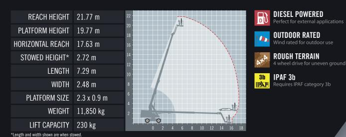
The Manitou 220TJ telescopic boom has a large platform that can hold up to 2 operators or 230 kg.
